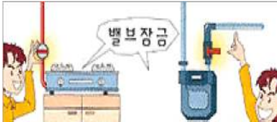
1. Lock the cock and the safety valve.
